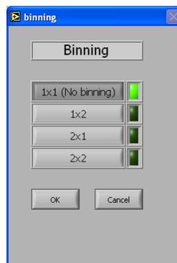
Figure 13: Window for binning the CCD.
