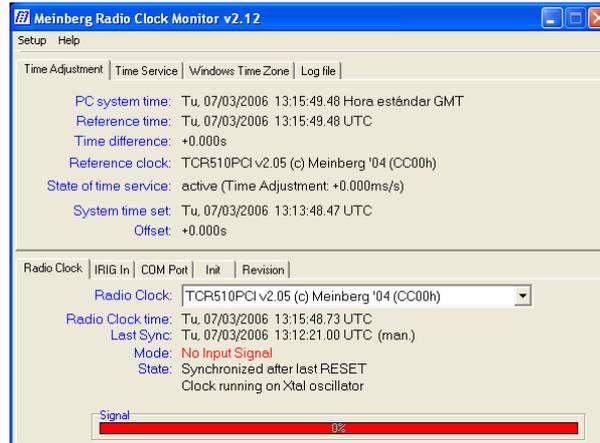
Figure 2: GPS interface when the system has not input signal
