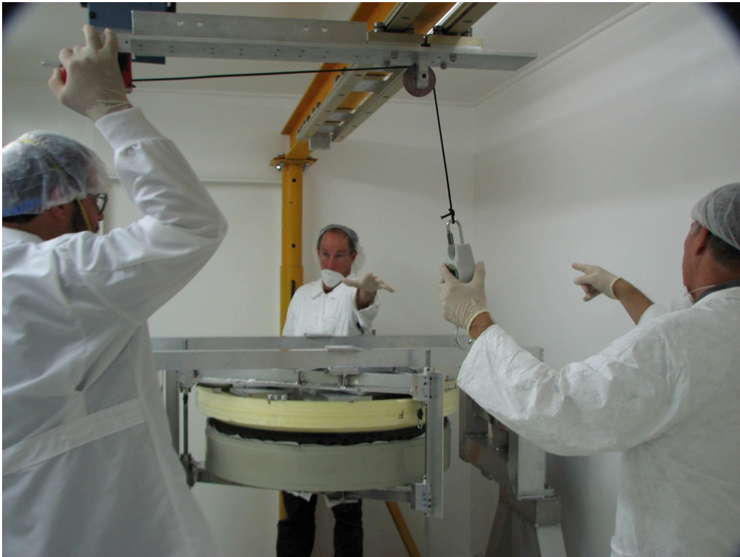
Figure 2 - Handling of one of the thin shells for coating. At this stage the the thin shell is clamped between two supports. From left to right: M. Wagner, M.J. Lefebvre and R. Sosa.
