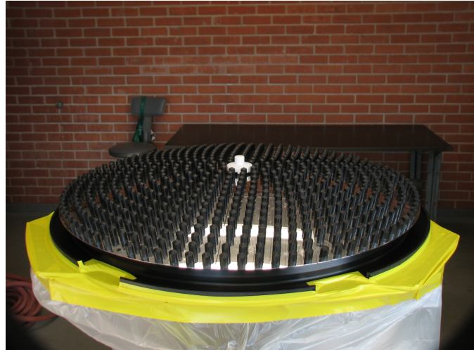
Figure 5 – Design of the magnet cover (left), the magnet used as counter-magnet to the magnet on the shell as well as the O-ring used to seal the cavity in which the shell’s magnet is housed are shown. (Right) Thin shell #3 ready to have the magnet side stripped and cleaned, 672 magnet covers have been installed on its surface.
