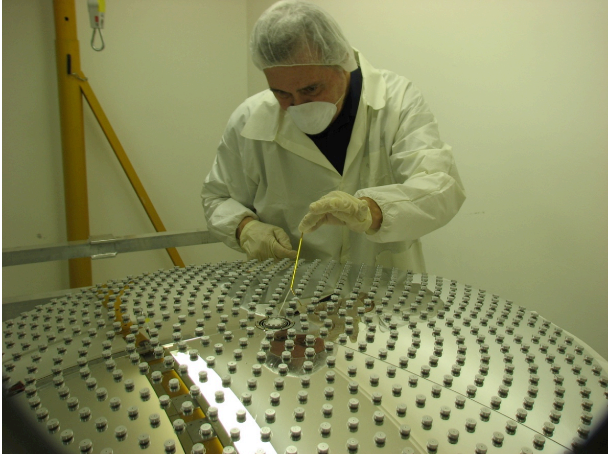
Figure 8 Thin Shell #3 after re-coating of its magnet-side. R. Sosa is removing some Kapton tape strips used to locally mask the coating and produce the necessary division lines in the coating layer.
