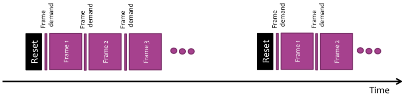
Figure 10: Bursts of multiple non-destructive reads.
