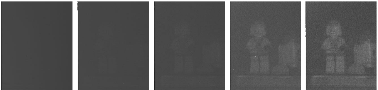
Figure 8: Low light scene imaged with gains of 1,6,13,45 and 90 (from left to right) showing only a few defective pixels at high gain (<10 defective pixels) on our engineering grade device, CDS readout at 1700 FPS.
