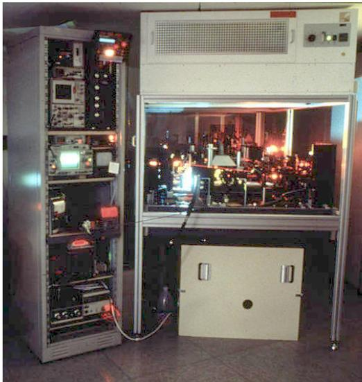
50W CW mode-locked *solid-state laser*
