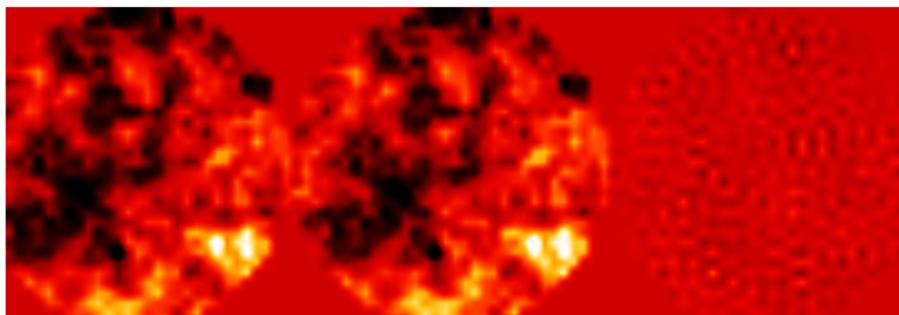
Simulated wave-front, reconstructed wave-front, 100×difference
