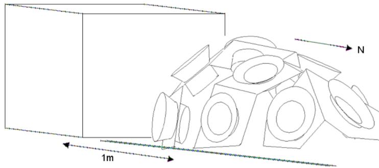
**Fig 1.** Drawing of PASS experiment (here with 10 cameras) in front of its enclosure, giving an approximate indication of the experiment's layout and size.
