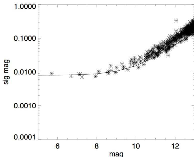
**Fig. 7.** Crosses indicate the rms error found in time-series photometry on the artificial stars in 15 simulated images similar to those shown in Fig. 6a. The solid line is identical to the solid line in Fig. 5 and indicates the total expected noise from S/N calculations. Some stars have photometric errors ‘better’ than the theoretical value; this is a result of the small sample of only 15 images.
