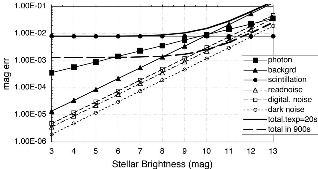
**Fig. 5.** Noises of the PASS instrument against stellar magnitude, as expected in star-trail images. The fat dashed line is the total noise for 900 seconds of integration, whereas all other lines indicate noises in a single 20 second exposure of a field at the celestial equator with the ‘base-line’ set-up (see text). Photometric precision suitable for transit-detection can be expected up to 10.5–11mag.
