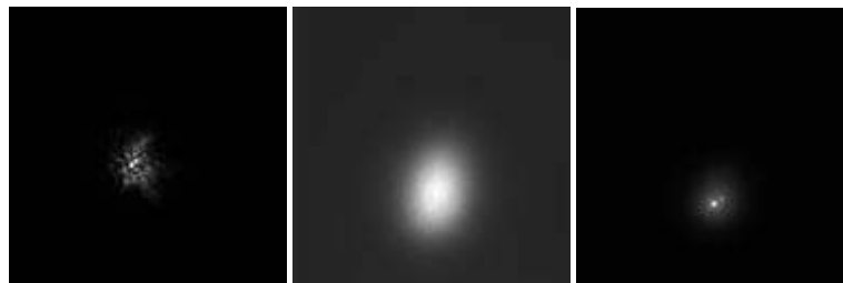
Fig. 5. Left: a 30ms exposure. Centre: natural seeing. Left: 1% of 4,000 aligned and averaged images.
