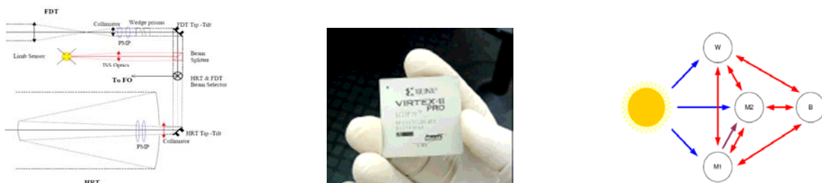
Figure 11: Left: Present concept of VIM that includes LCVRs (PMP). Center: prototype FPGA of the Stokes inversor. Right: Nodes of the thermal model of VIM.
